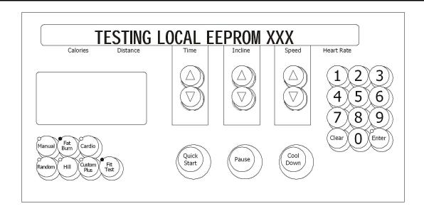
This test allows the user to test the display console EEPROM. This test will read/write/replace all used locations in the display console EEPROM. The EEPROM location being tested will be displayed in the heart rate window. If there is an error, the bad location will be displayed.
